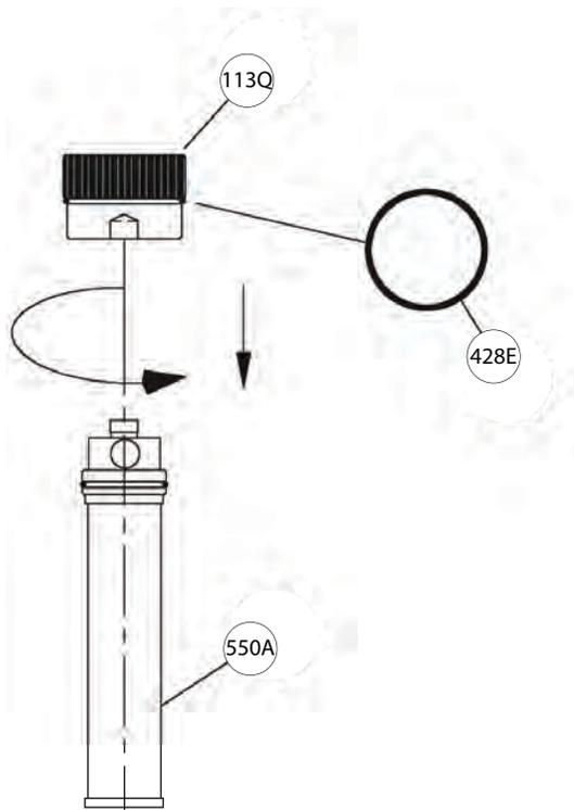
**Figure 34: Oil filter replacement**
