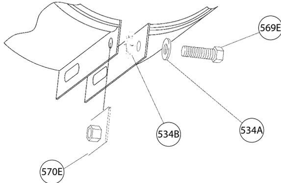
**Figure 25: Coupling guard hardware installation**
