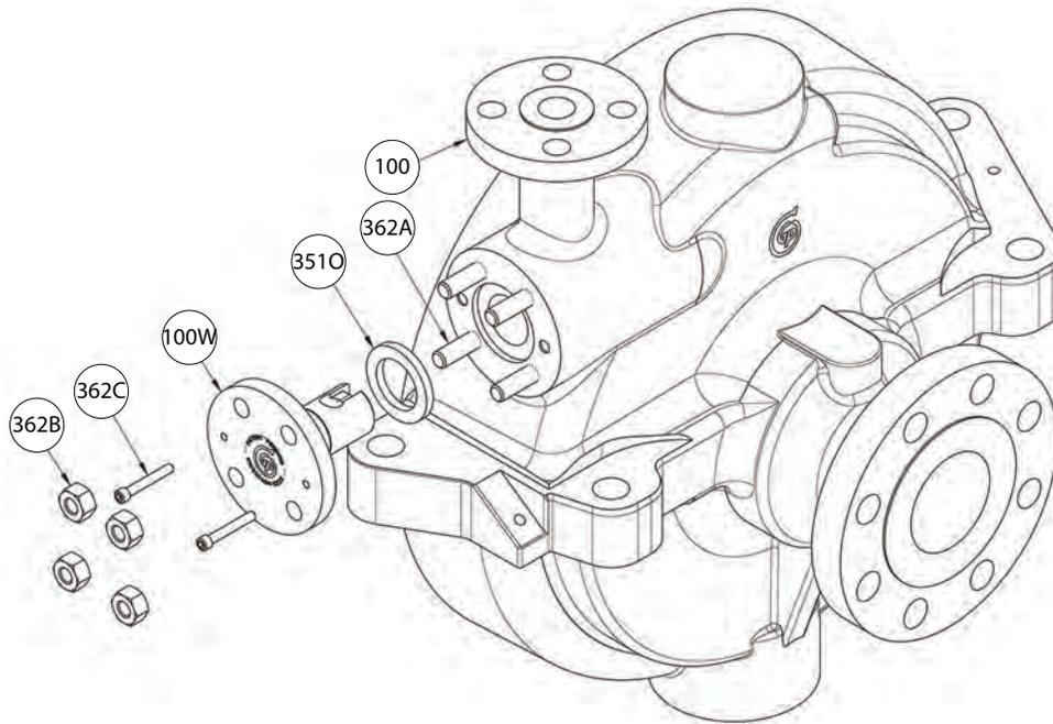
**Figure 47: Venturi insert removal**
