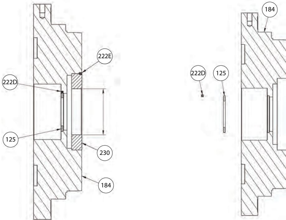
**Figure 63: Seal chamber cover wear ring and throat bushing**
