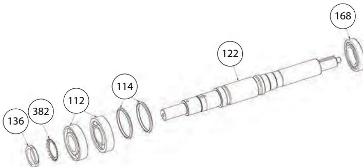
**Figure 52: Shaft and bearing removal**
