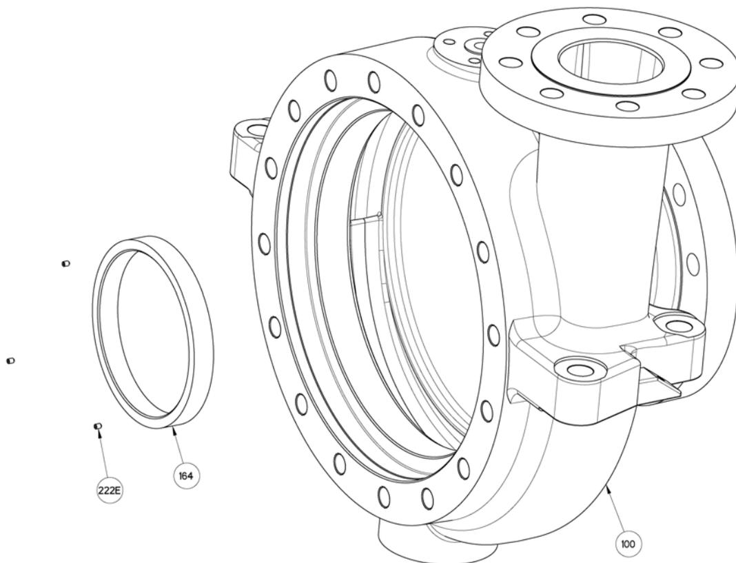
**Figure 62: Casing wear ring**
