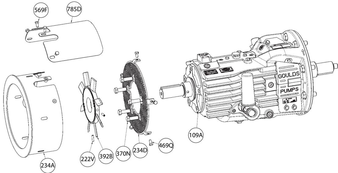
**Figure 49: Power end disassembly**
