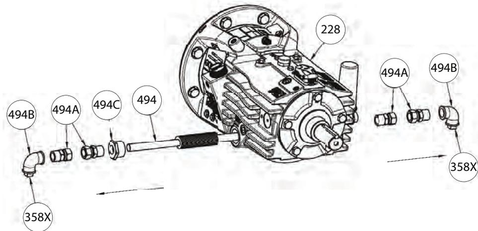
**Figure 51: Frame cooling removal**
