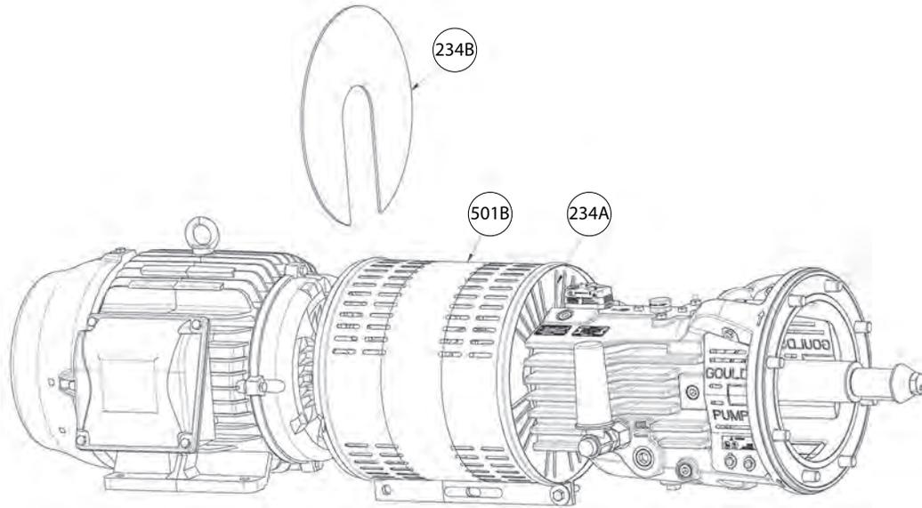
**Figure 27: Coupling guard motor end plate**
