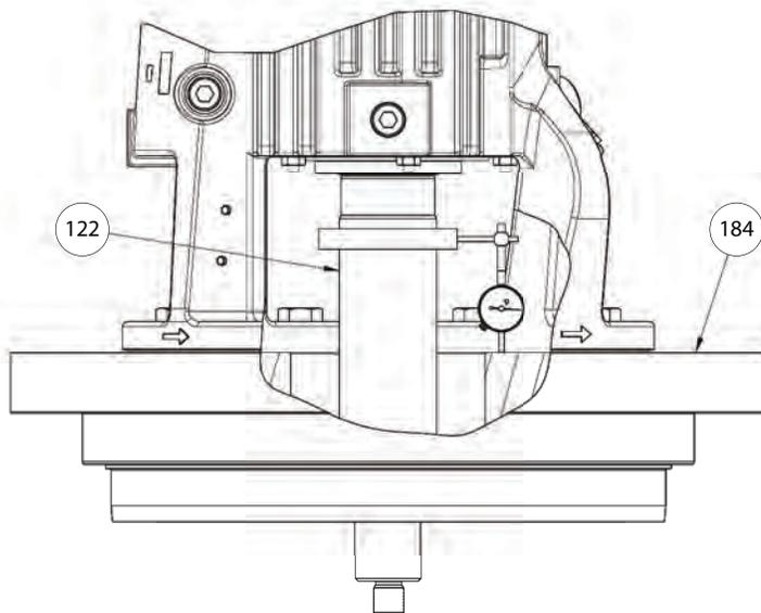
**Figure 77: Seal-chamber face runout**
