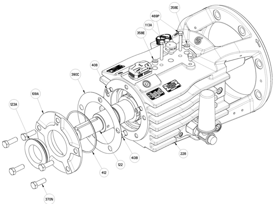
**Figure 70: Shaft and bearing frame assembly**
