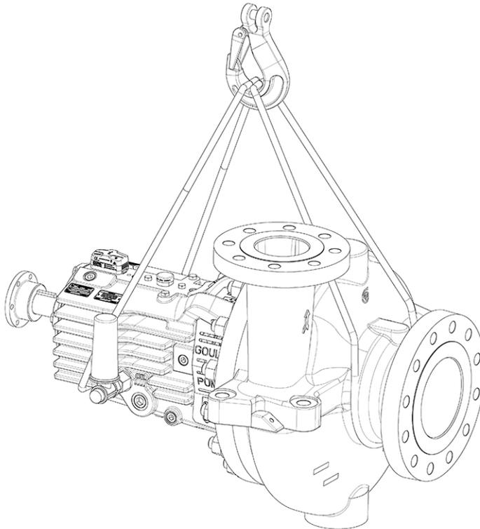
**Figure 3: Example of a proper lifting method of pump with driver**
