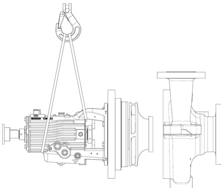
**Figure 81: Back pull-out assembly**
