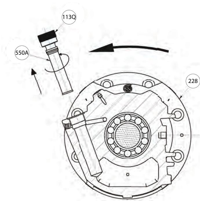
**Figure 33: Oil filter assembly removal**
