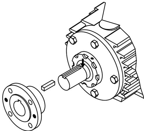
Figure 80: Coupling hub installation
