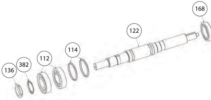
**Figure 67: Radial (inboard) bearing installation**
