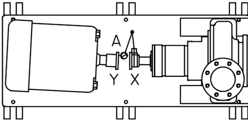
**Figure 17: Example of incorrect horizontal alignment (top view)**
