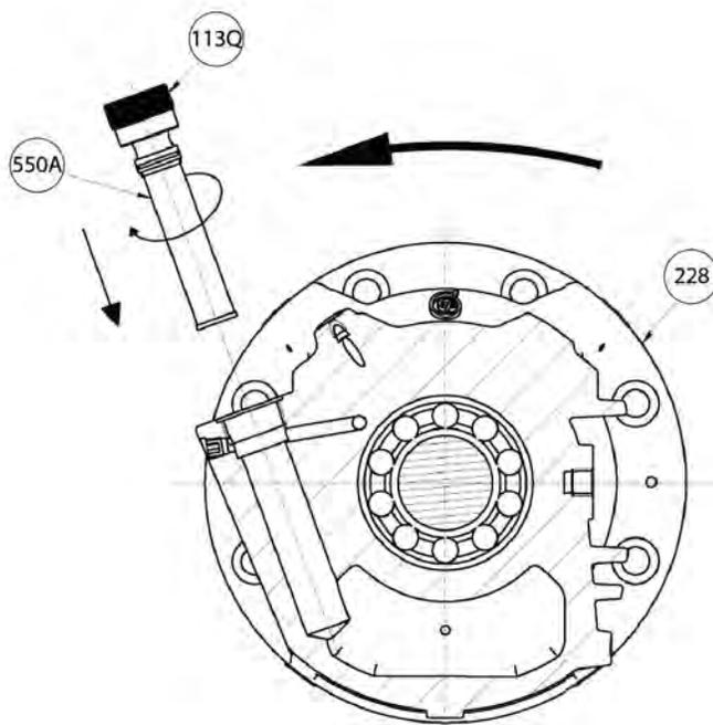
**Figure 36: New filter installation**
