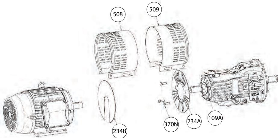
Figure 21: Coupling guard removal
