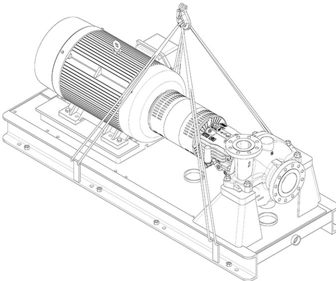
**Figure 5: Example of a proper lifting method of pump on base plate with driver and motor**
