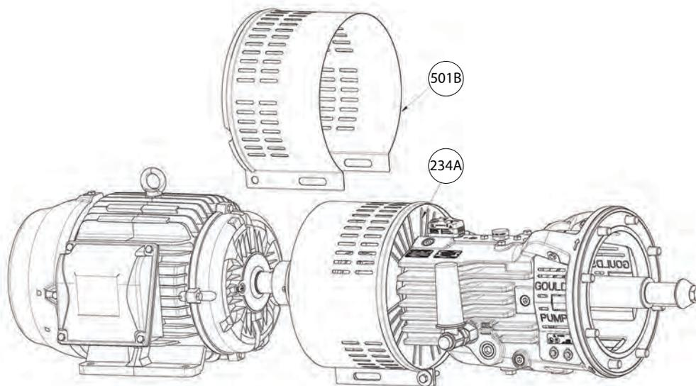
**Figure 26: Coupling guard motor**
