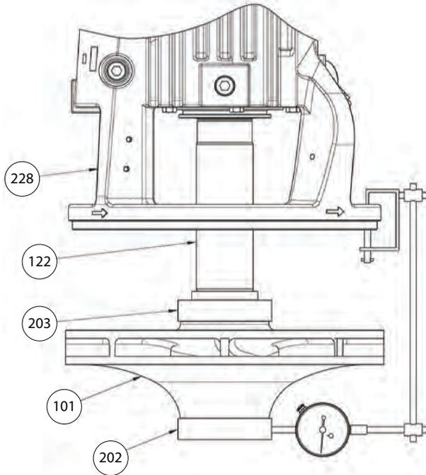
**Figure 65: Impeller wear-ring runout**
