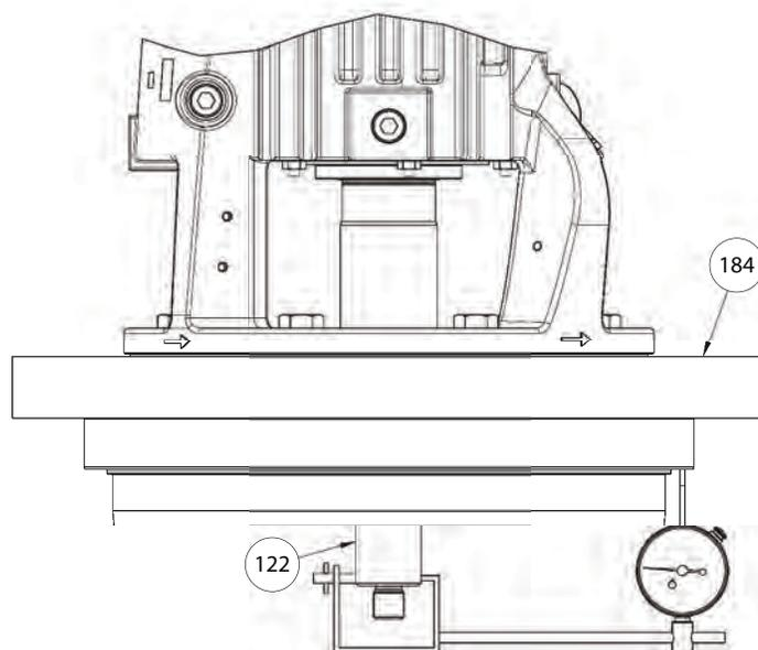
**Figure 74: Seal-chamber cover face runout**
