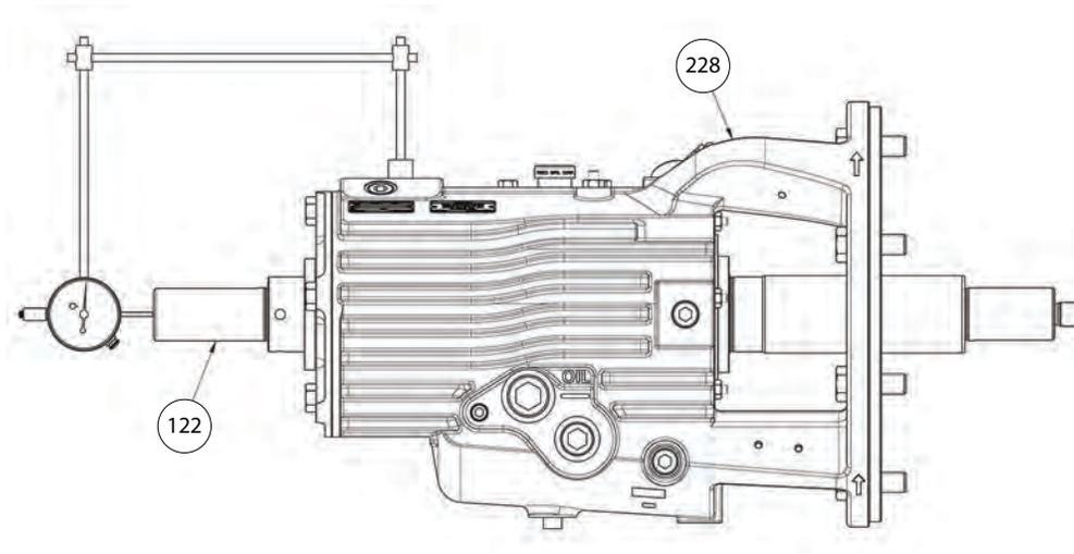
**Figure 72: Axial end play determination**
