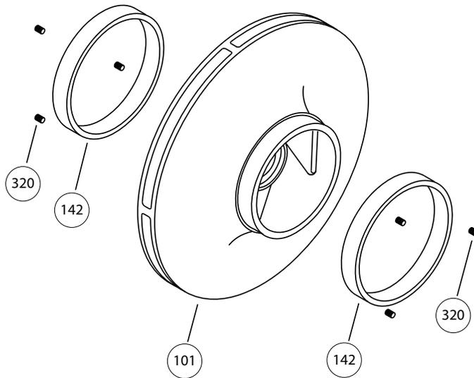
**Figure 61: Replace impeller wear ring**
