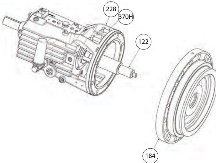
**Figure 73: Seal chamber cover**
