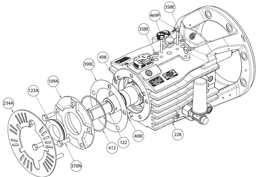
**Figure 50: Thrust cover removal**
