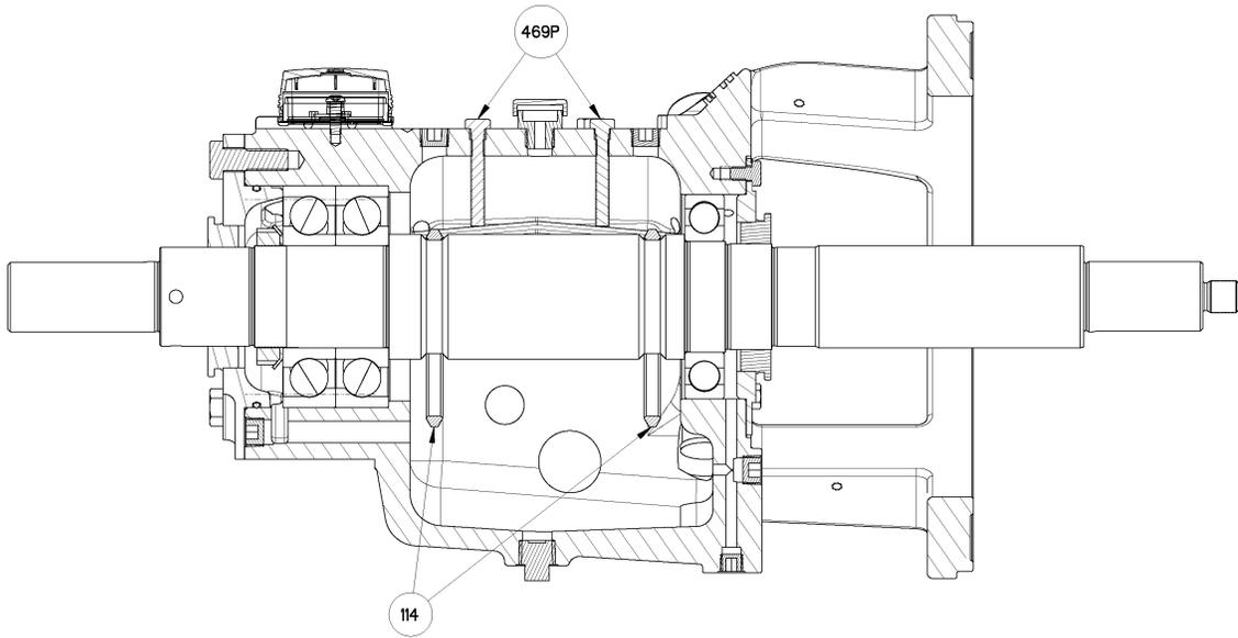
**Figure 31: Frame/shaft/rings in proper location**
