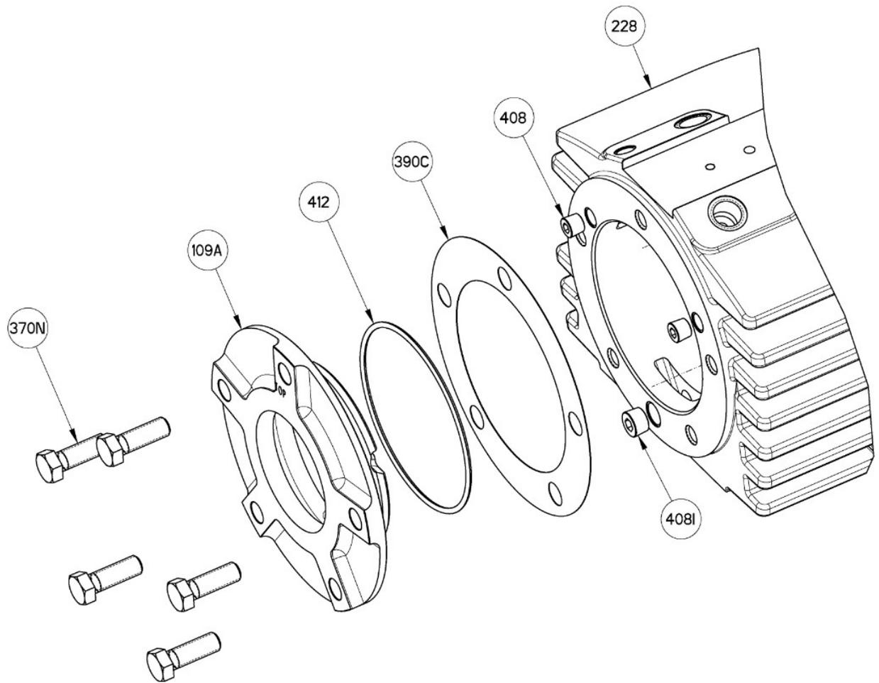
**Figure 71: Bearing frame assembly**
