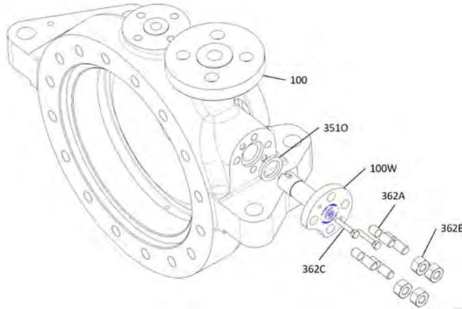
**Figure 82: Venturi insert and casing**
