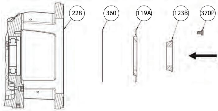
**Figure 69: Radial bearing isolator installation for 13i frame only**
