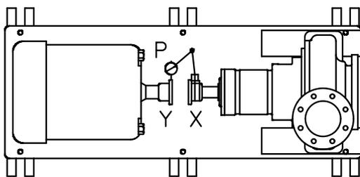
**Figure 19: Example of incorrect horizontal alignment (top view)**
