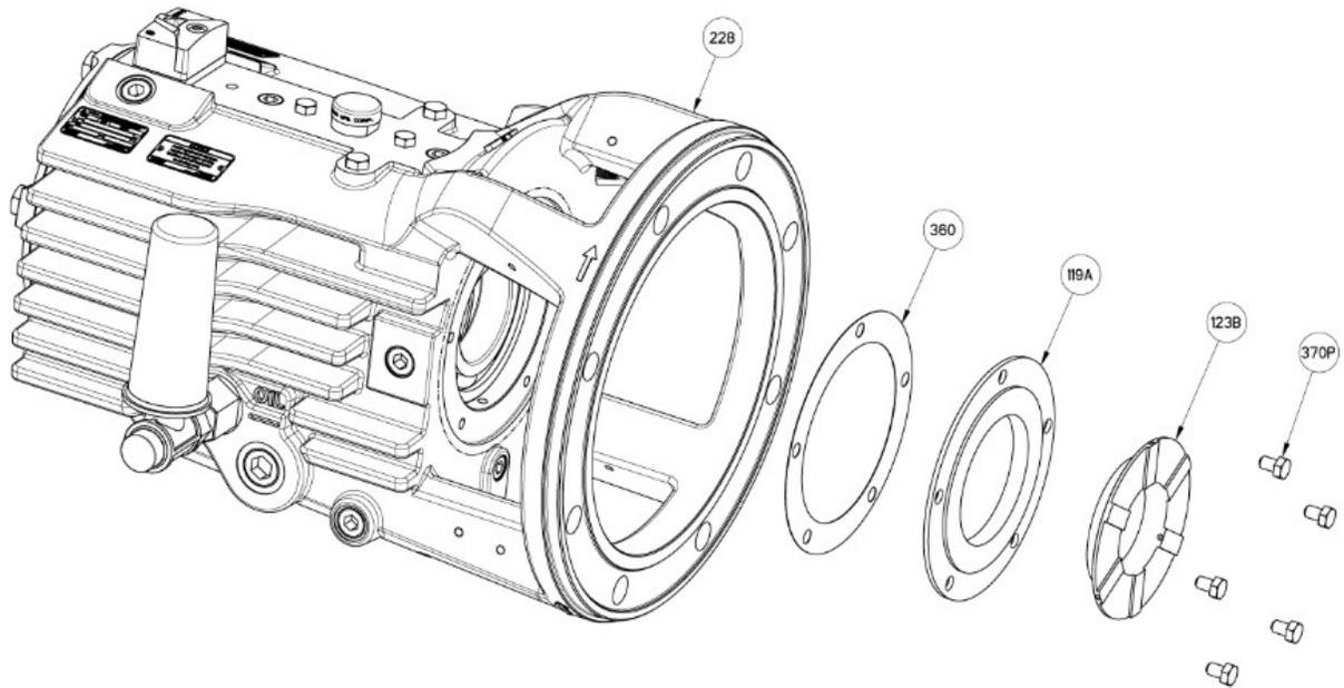
**Figure 30: Install the Air Cooling Package - Radial heat flinger**
