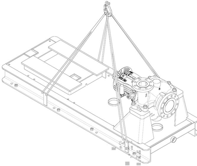
**Figure 4: Example of a proper lifting method of pump and driver on base plate**
