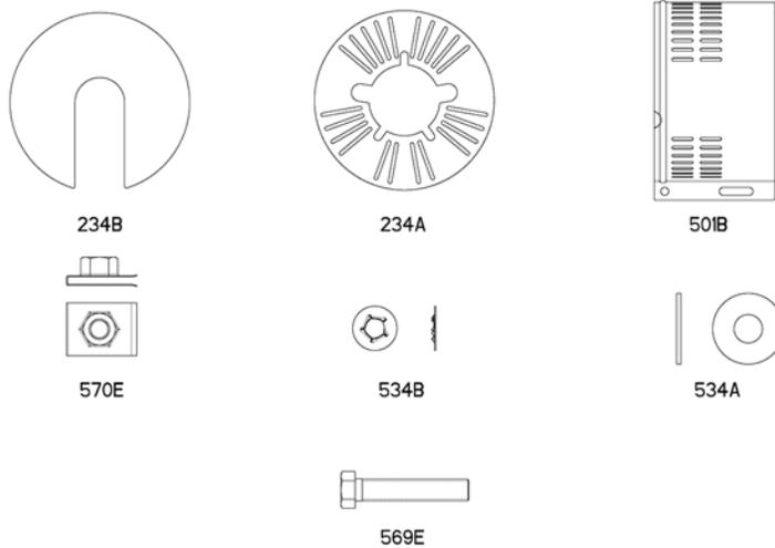
**Figure 22: Coupling guard required parts**
