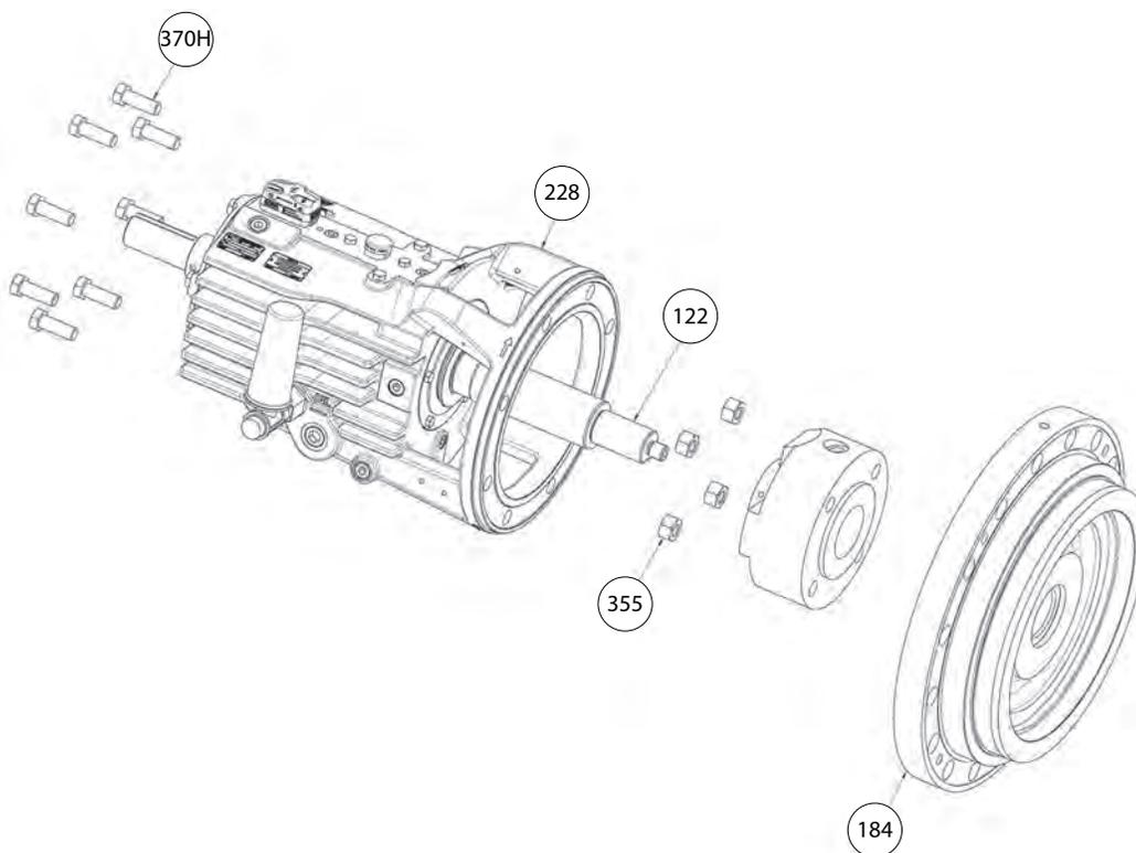
**Figure 48: Seal-chamber cover removal**
