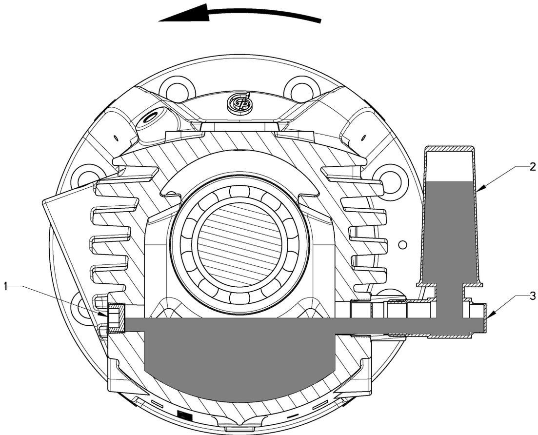
**Figure 32: Checking oil level**
