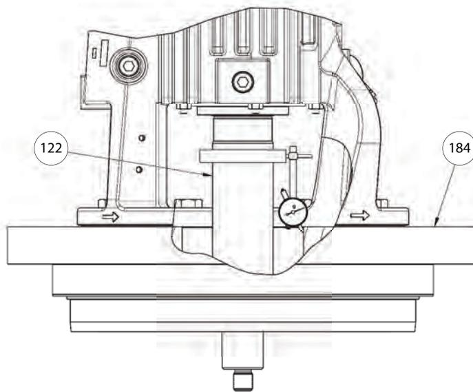
**Figure 78: Seal-chamber lock (register) runout**
