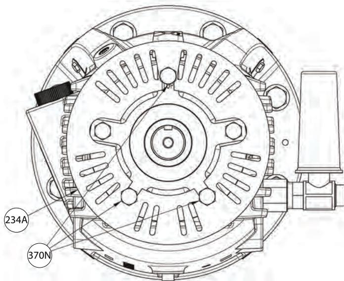
**Figure 23: Thrust bearing end cover removal**
