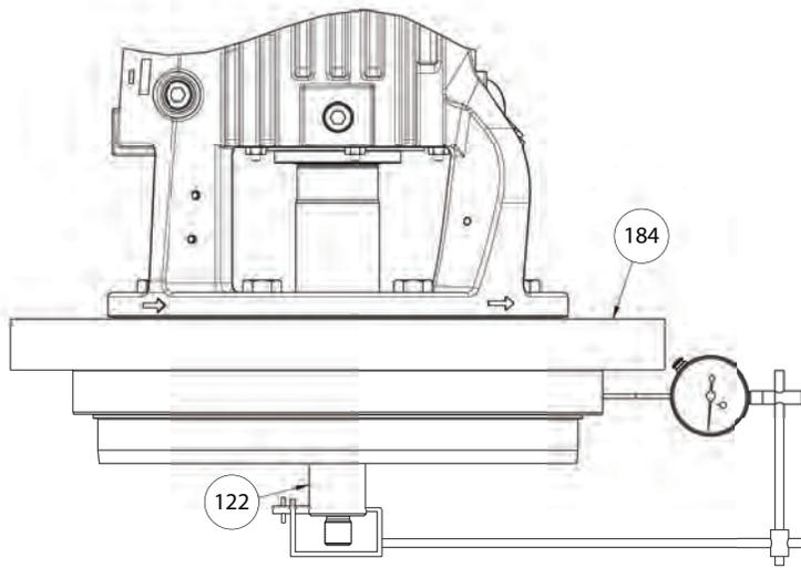
**Figure 75: Seal-chamber cover lock runout**
