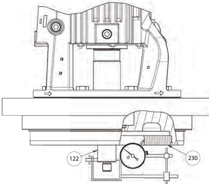
**Figure 76: Seal-chamber cover wear-ring runout**
