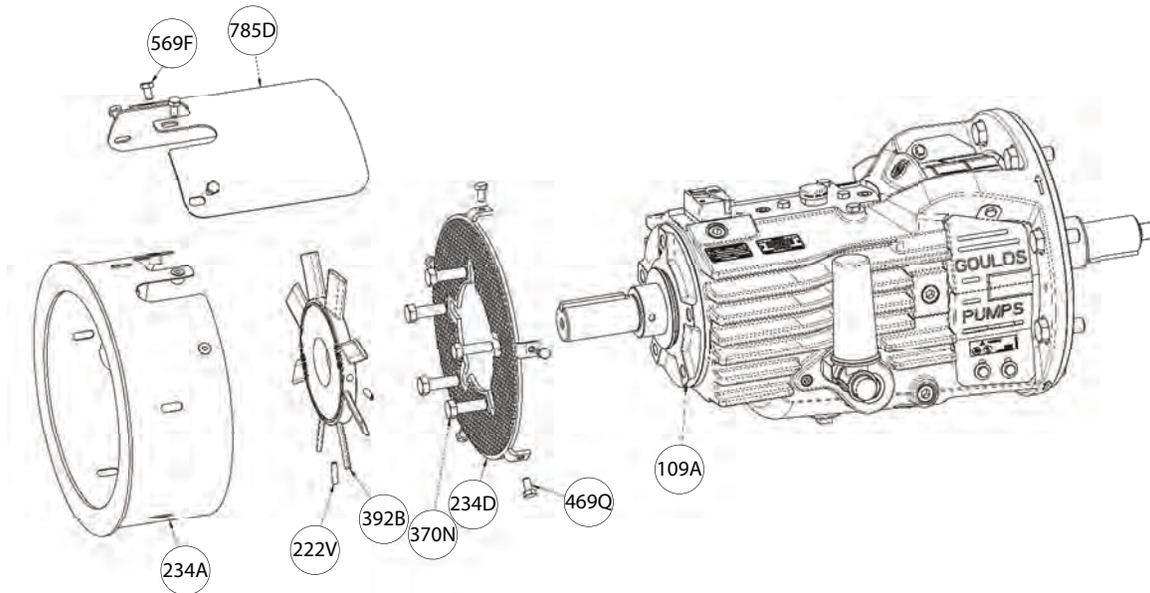
**Figure 29: Install the Forced Convection Cooling (As required)- Cooling Fan, Guards and Cowling**
