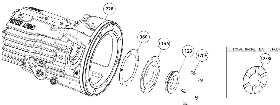
**Figure 68: Bearing frame**
