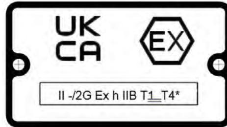
Figure 2: Typical UKCA Ex nameplate
