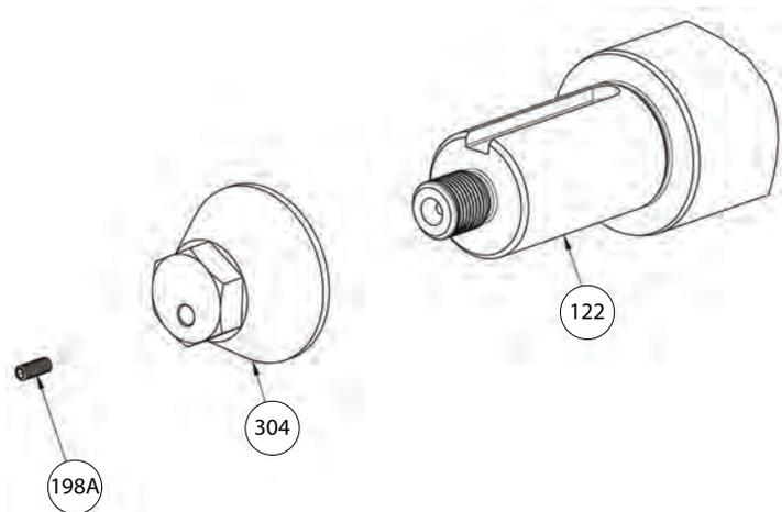
**Figure 46: Impeller removal**
