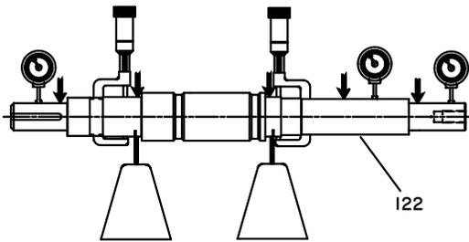
Figure 57: Shaft inspection
