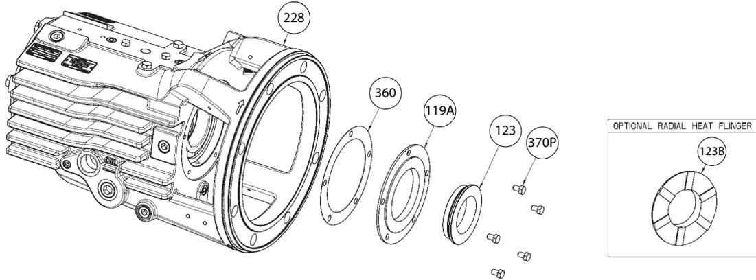
**Figure 53: Radial bearing isolator or optional radial heat flinger removal**
