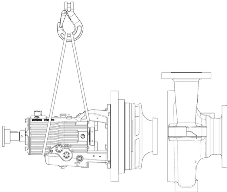
**Figure 45: Lifting sling through bearing frame**
